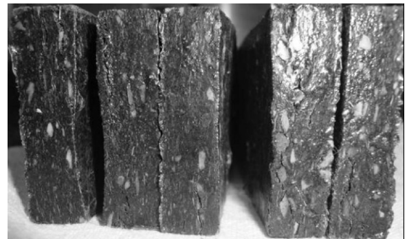
Fig. 9. Modification of physical behavior of composites after aging test.
